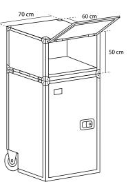
fully pull-out and detachable drawer (self-closing mechanism)
